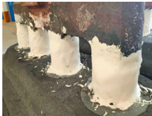
Figure 2. Application of anti-oxidation coating.
